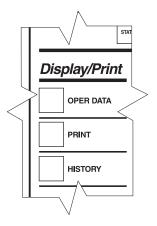
The Display/Print keys allow the user to retrieve system and unit information that is useful for monitoring unit operation, diagnosing potential problems, troubleshooting, and commissioning the unit.
