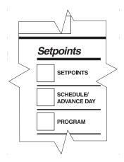
Programming and viewing the cooling and heating setpoints, daily schedule, and safeties is accomplished by using the 'SETPOINTS' keys.
