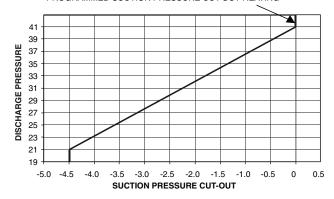
At a discharge pressure of 41 barg and above the actual suction pressure cut-out equals the programmed suction pressure cut-out heating. As the discharge pressure fall below 41 bar to a minimum of 21 bar the programmed suction pressure cut-out heating is lowered lineally by a maximum of 4.5 bar. Below a discharge pressure of 21 bar the actual suction pressure cut-out is equal to the programmed suction pressure cut-out heating minus
