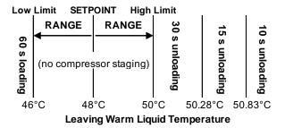
Each system has its own anti-recycle timers. The anti-recycle time under the PROGRAM key can be programmed between 240 and 600 seconds and sets the minimum start-to-start time of the lead compressor in a system. Due to lead lag rotation in a system, consecutive lead compressor starts are not with the same compressor. A second non-programmable anti-recycle timer, stop to start is fixed at 90 seconds, starts to countdown when the lead compressor in a systems cycles off.
