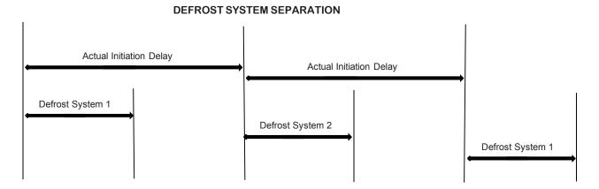
As it can be seen from the table in determining if a change should take place in the initiation delay the priority is given to the system with the most frost. The defrost of each system are spaced equally apart as shown in the Defrost System Separation figure.
