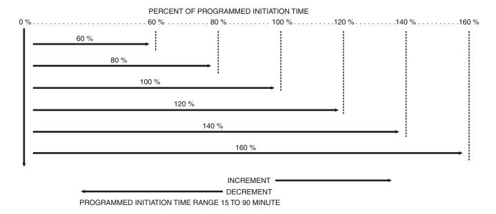
If the termination temperature is not reached within 200% of the termination delay setting, a time override occurs and the defrost is terminated and the initiation delay reduced by 20%.
