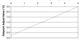
Any adjustment value in excess of the value taking the Setpoint Low Limit to 40°C is added to the Setpoint High Limit. When the run time exceeds 5 minutes the 'Setpoint Adjust Value' returns to zero. This will occur whilst the unit is running. Pressing the 'SETPOINTS' key seven times will display the lead system's last run time and the 'Setpoint Adjust Value'.
