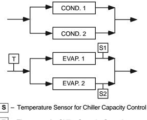
**T** – Thermostat for Chiller Capacity Control
