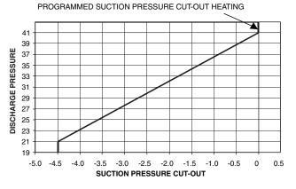
At a discharge pressure of 41 barg and above the actual suction pressure cut-out equals the programmed suction pressure cut-out heating. As the discharge pressure fall below 41 bar to a minimum of 21 bar the programmed suction pressure cut-out heating is lowered lineally by a maximum of 4.5 bar. Below a discharge pressure of 21 bar the actual suction pressure cut-out is equal to the programmed suction pressure cut-out pressure cut-out heating minus
