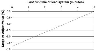
Any adjustment value in excess of the value taking the Setpoint Low Limit to 40°C is added to the Setpoint High Limit. When the run time exceeds 5 minutes the 'Setpoint Adjust Value' returns to zero. This will occur whilst the unit is running. Pressing the 'SETPOINTS' key seven times will display the lead system's last run time and the 'Setpoint Adjust Value'.
