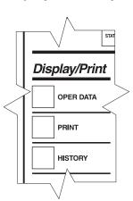
The Display/Print keys allow the user to retrieve system and unit information that is useful for monitoring unit operation, diagnosing potential problems, troubleshooting, and commissioning the unit.
