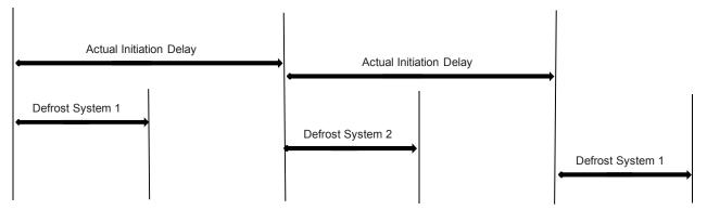
As it can be seen from the table in determining if a change should take place in the initiation delay the priority is given to the system with the most frost. The defrost of each system are spaced equally apart as shown in the Defrost System Separation figure.
