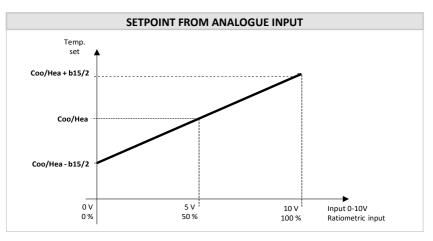
Correction calculation with ratiometric input (b20=1):
