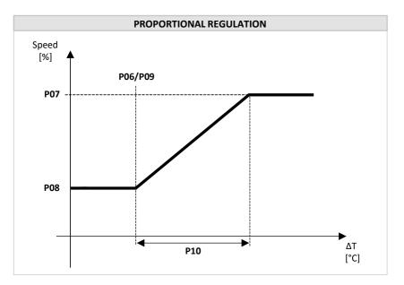
In practice, in cooling mode, if the temperature difference between the inlet and outlet is greater than P09 + P10, the circulator runs at maximum speed, but if the difference is less than P09 - 0.2°C, it runs at minimum speed; in the remaining cases, the pump modulates the speed proportionally. In heating mode, the same considerations apply, replacing parameter P06 with parameter P09. In sanitary production the circulator always runs at maximum speed.
