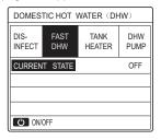
Use " 🖰 " to turn on/off "CURRENT STATE" of FAST DHW function.
