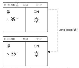
The controller will be locked if it has not been operated for a long time (about 120 seconds). If the controller is unlocked, long press " &", the controller will be locked.
