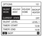
Use " ♥" to turn on/off current state of SILENT MODE, Timer1 and Timer2, use "♥", "▲" to select the silent level and adjust the start/end time of the timer.
