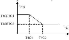
State: In the setting of the wired controller, if T4C2<T4C1, then exchange their value; if T1SETC1<T1SETC2, then exchange their value. (T1SETC1, T1SETC2,T4C1,T4C2 can be set in "FOR SERVICEMAN" .)
