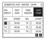
Use " $\blacktriangleleft$ ", " $\blacktriangleright$ ", " $\blacktriangleright$ ", " $\blacktriangle$ " to scroll and use " $\blacktriangledown$ ", " $\blacktriangle$ " to adjust the start time, press " $\rightharpoonup$ " to select the timer.
