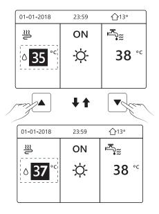
The operation methods of adjusting the temperature in other menus (including that the unit has no DHW function or DHW mode is set unavailable) is similar.
