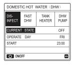
Use " <sup>(t)</sup> " to turn on/off "CURRENT STATE", and use" ▼", "▲" to adjust the operate date and start time of disinfect function.
