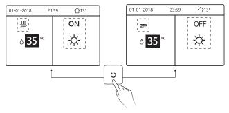
The operation methods of turning on or off the operation mode in other menus is similar.
