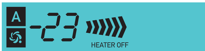
Figure 7. LCD display when the device is under automated control of MagicAir system (section 5.4), heater is off or not installed in this configuration
