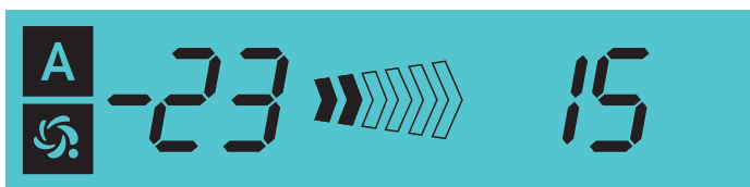
Figure 4. LCD display, when the device is under automated control of MagicAir system (section 5.4):
