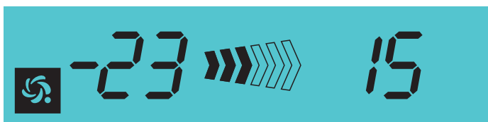
Figure 5. LCD display when the device is connected to MagicAir system (section 5.4), but remains under manual control
