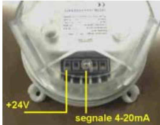
Figure 24: terminal board of the differential pressure switch.
