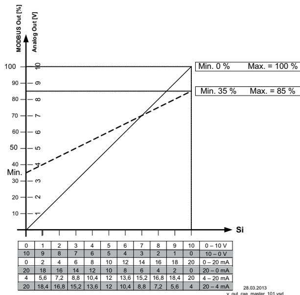
MODBUS Out: speed setting over MODBUS
