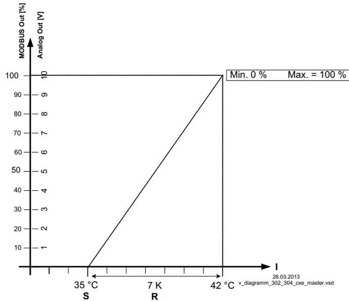
MODBUS Out: speed setting over MODBUS
