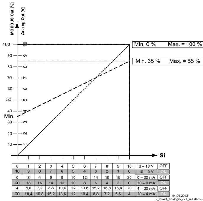
MODBUS Out: speed setting over MODBUS
