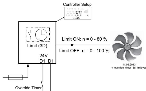
Contact depending on device type at terminals “D1” - “D1” or “D1” - “24 V”
