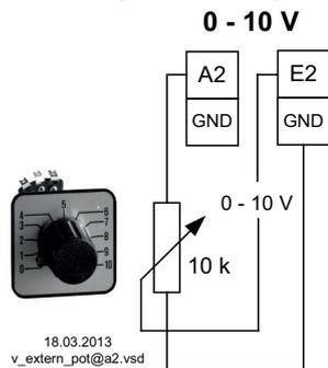
**External Setpoint** via external signal instead of “Setpoint 1”. The “external Setpoint” function must be activated in base setup [1E] for “E3 function”. The active external Setpoint value is displayed in the “info” menu group.
