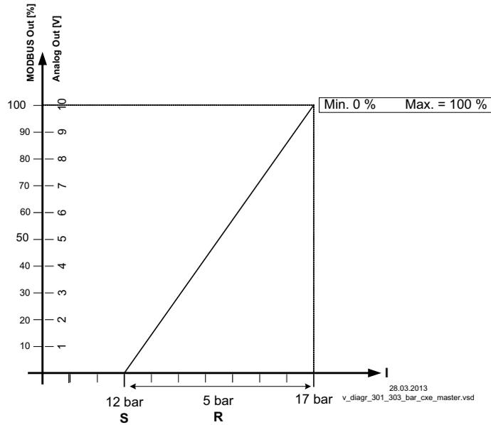
MODBUS Out: speed setting over MODBUS
