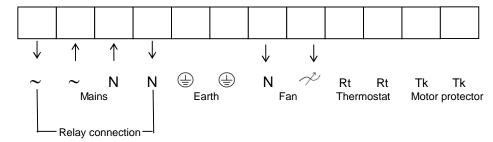
Relay connection: There is always 230V between ~ and N when the transformer knob is in one of the positions 1-5. If the motor protection is not in use, Tk shall be looped together.
