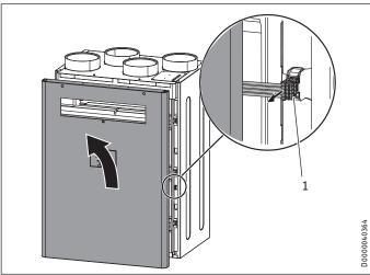
1 Plug on cable from programming unit to appliance
