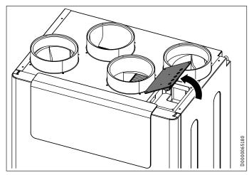
► Carefully lift up the control panel cover. The terminal block, from which cables lead into the appliance, is suspended from the underside of the cover.
