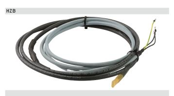
Self-limiting flexible ribbon heater to keep the condensate connection for air I water heat pumps free of ice. Both versions have a 2 m connecting cable. Heated length: HZB-1: 1 m; HZB-2: 2 m.
