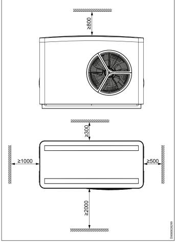
► Maintain the minimum clearances to ensure trouble-free operation of the appliance and facilitate maintenance work.
