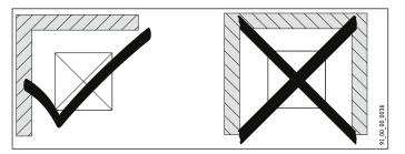
► Never install the appliance in a recess. Two sides of the appliance must remain exposed.
