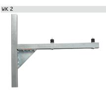
Corrosion-protected wall mounting bracket made from zinc-plated steel for on-site installation. Height adjustments can be made on the wall rail, while the appliance rail provides the possibility to align the appliance. Standard delivery includes: 2 pce incl. anti-vibration mounts and 2 m self-limiting ribbon heater.
