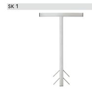
Stainless steel, T-shaped support for floorstanding, concrete-embedded installation. Standard delivery includes: 2 pce incl. installation aid for a defined clearance dimension, anti-vibration mounts, plus 1 m self-limiting ribbon heater.
