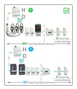
In example 2 and 3, the PowerTag energy sensors or PowerTag control modules are not balanced between the two gateways.
