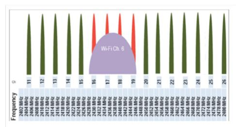
The frequency range associated to the selected channel in a gateway can be also used by another wireless system such as Wi-Fi network and third-party wireless equipment around it.
