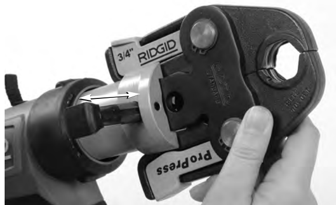
Figure 7 – Attachment Mounting Pin
