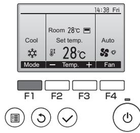
Press the [F1] button to go through the operation modes in the order of "Cool, Dry, Fan, Auto, and Heat."
