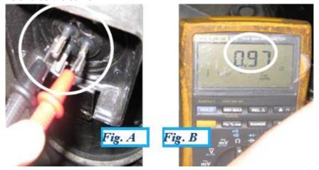
3.2 Measure the resistance between the compressor's U,V,W and GND respectively. The resistance should be more or less mega-Ohms.
