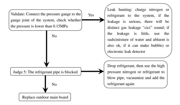
Remarks: When system appear P2 protection for 3 times in 30 minutes, system will auto shut down and display H5 malfunction, which can recover only by restarting the machine. Malfunction should be promptly treated to avoid further damage.
