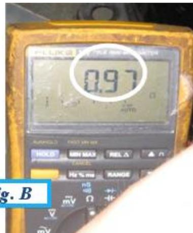
3.2 Measure the resistance between the compressor's U,V,W and GND respectively. The resistance should be more or less mega-Ohms.
