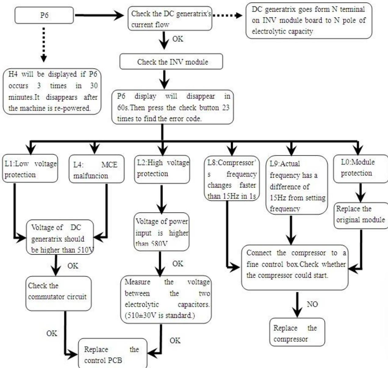
Detailed Malfunction Code of Module Protection (P6) (Only for 18kW)
