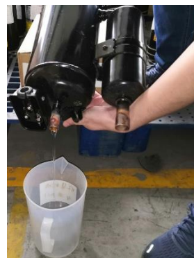
Figure 6-2.5: Draining oil from a compressor
