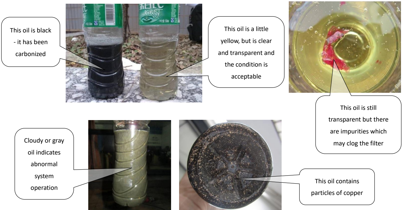
Figure 6-2.7: Inspecting compressor oil
