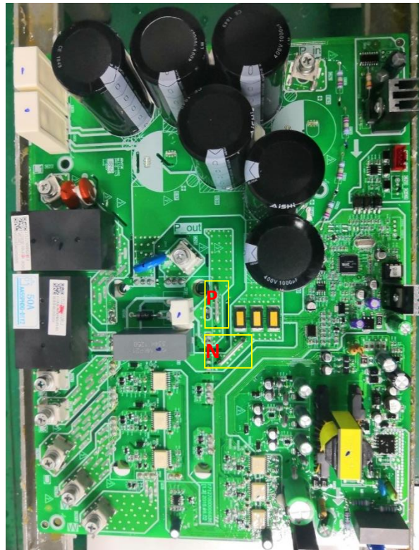
Figure 6-2.1: P and N terminals on Inverter module
