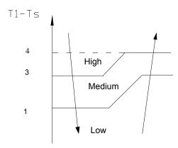
(3) Anti-freezing control to indoor evaporator in cooling mode
