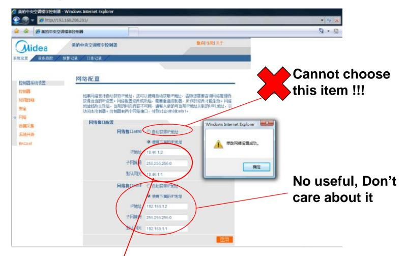
Change the ip address under the same address range. Pls ask the IT administrator which ip address is available. In this case, ip address of CCM08 have been changed to 10.46.1.2
