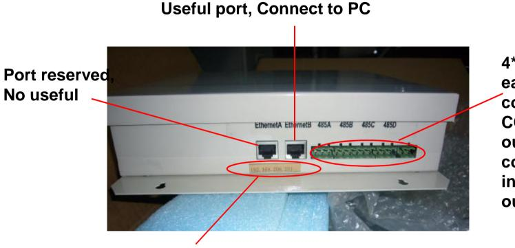
4\*Port RS485, each port connect one CCM(indoor or outdoor) and corresponding indoor or outdoor units
