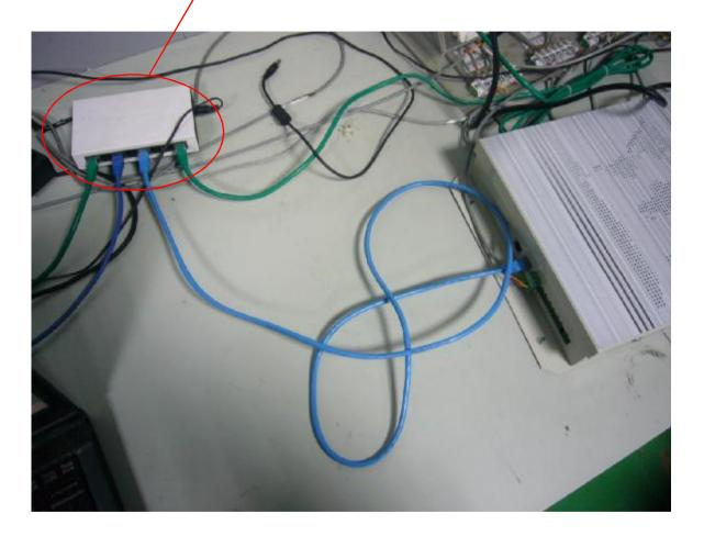
On any PC of LAN, input 10.46.1.2 on IE address bar, get into the web control interface, So CCM08 has been connected to LAN.
