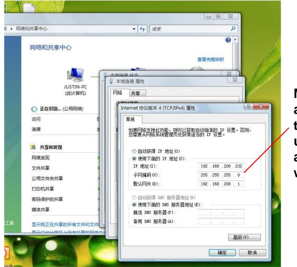
Modify the PC ip address to:192.168.208.232, under the same address range with CCM08.
