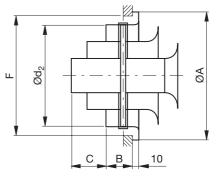
Diffused supply air - for installation in a wall or duct side. Remove the external pipe.
