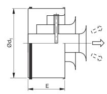
Diffused supply air - for installation in a circular duct or fitting. Supplied adapted to this form of installation as standard.
