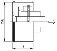
Concentrated supply air - for installation in a circular duct or fitting. The insert is turned 180 degrees.
