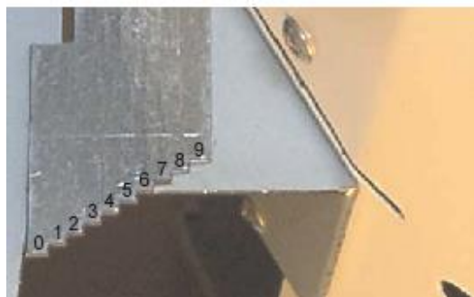
Step indicators showing the position of each regulating screw.
