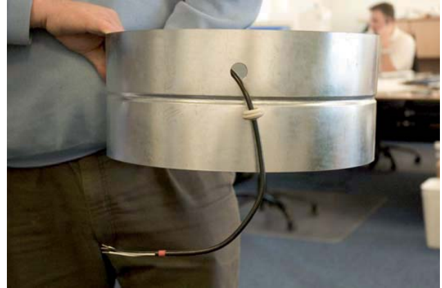
Cable lead-in is mounted on electric cable.
