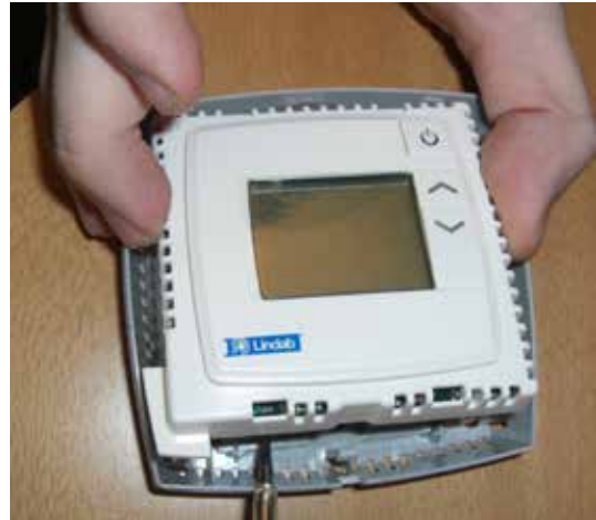
2. Remove the front including the circuit board
