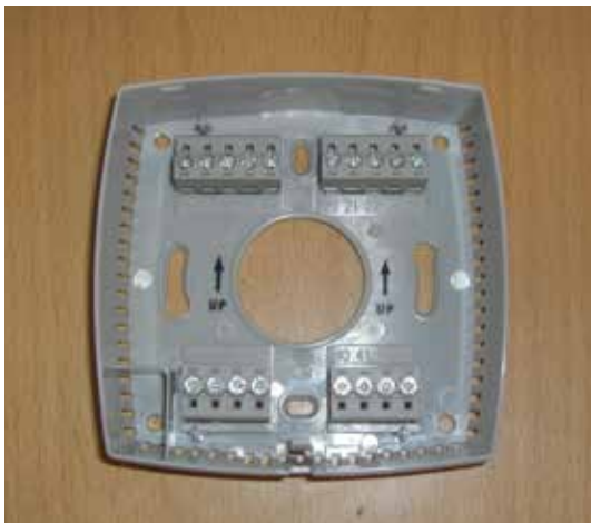
3. Mount the bottom plate on electrical box or directly on the wall
