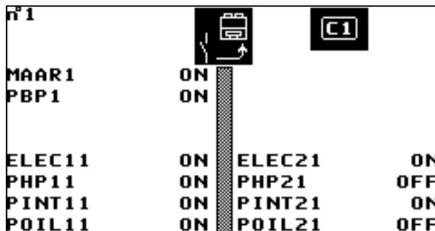
This screen shows the state of all the logic inputs associated with the circuit and its compressors.
