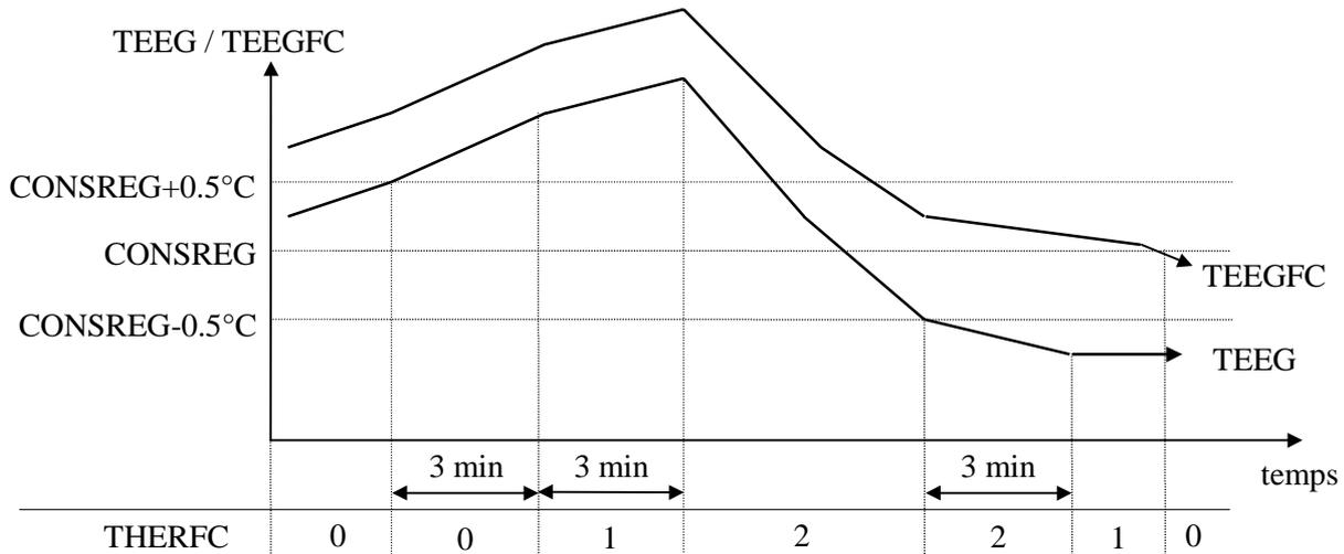
The thermostat is incremented by one stage if TEEG remains greater than  $\text{CONSREG}+0.5^{\circ}\text{C}$  for over 3 minutes. As long as this condition on TEEG is satisfied, THERFC continues to be incremented by one stage every 3 minutes.
