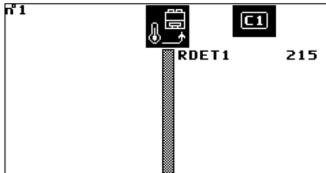
This screen shows the analogue inputs for the refrigerant circuit which are not shown in the refrigerant diagram screens described in § 3.5. (e.g. opening of electronic expansion valve).
