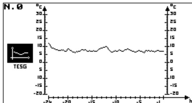
The monitoring frequency for the temperature of chilled water output (or hot water for a PAC) is 10 minutes, over a complete 24 hour cycle. The console therefore memorises the last 144 values of the monitored variable.
