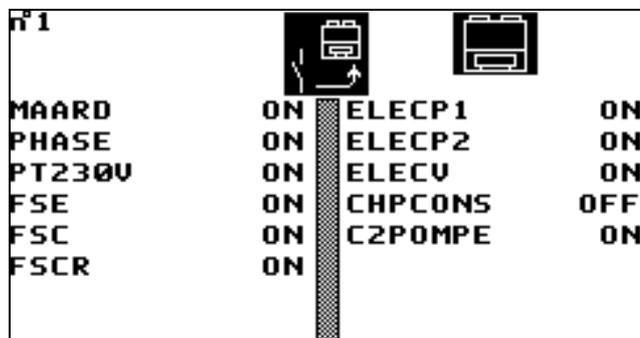
This screen shows the states of contacts which have an effect on the overall operation of the machine (e.g.: remote on / off, circuit breakers for pumps, choice of setting instruction, etc.)
