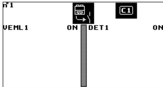
This screen displays the state of the actuators which control circuit components other than the compressors, whose operation has already been described in operating states for circuits (see § 3.4.).
