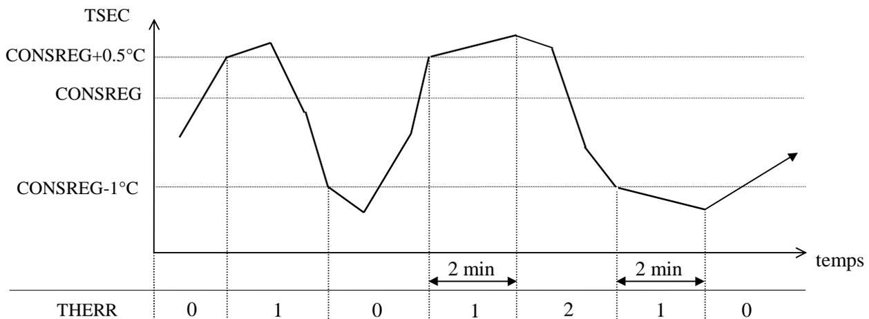
As soon as TSEC becomes greater than  $\text{CONSREG} + 0.5^\circ\text{C}$ , capacity is reduced. As long TSEC remains above  $\text{CONSREG} + 0.5^\circ\text{C}$ , an additional capacity reduction cuts in (if applicable) every 2 minutes.
