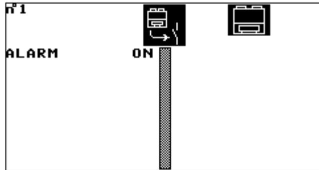
This screen displays the state of the actuators which control machine components other than those already described in operating states for circuits and pumps (e.g. general alarm).
