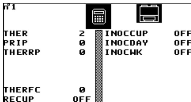
This screen gives the values of calculated variables which apply to the entire machine. (e.g.: priority status for pump operation, pump operation, idle functions, etc.)
