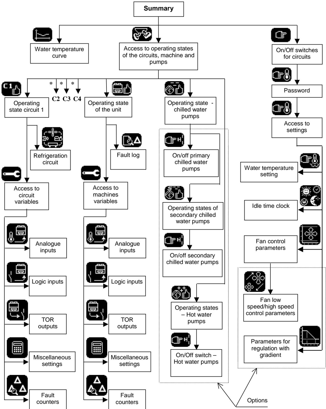
\* For units with more than one refrigeration circuit, branches C2, C3 and C4 corresponding to operating states for circuits no. 2, 3 and 4, are active.
