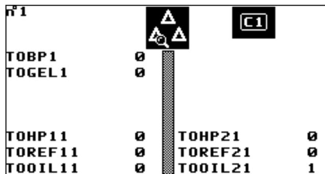
This screen shows the values of counters for all faults on the circuit and its compressors.
