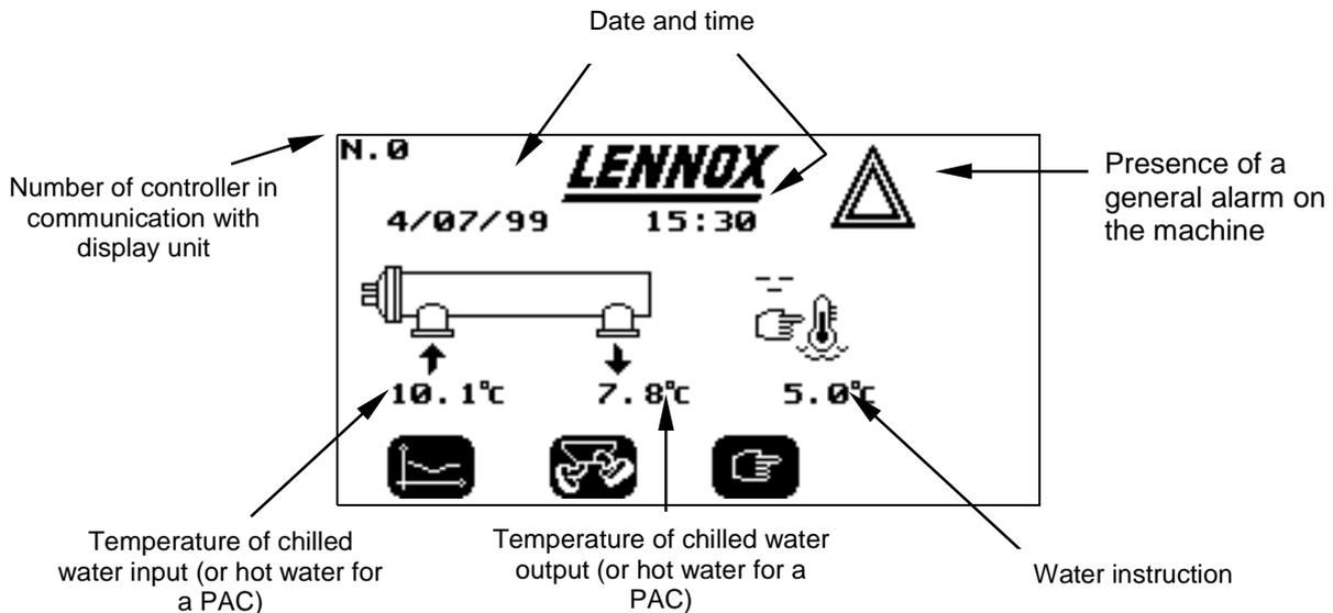
On a machine not fitted with the option "regulation with gradient", the active water instruction (CONSEA or CONSEB) is a variable which can be modified in "modification" mode. In the case of regulation with gradient, the active instruction CONSEA can be modified. However CONSALC cannot be modified, since it is the result of a calculation (see pages 15 and 16).
