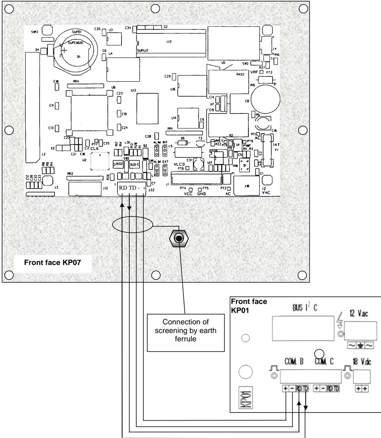
The cable connecting the display unit to the principal unit must be earthed by means of an earth ferrule fixed to the front face using the nut provided for this purpose.
