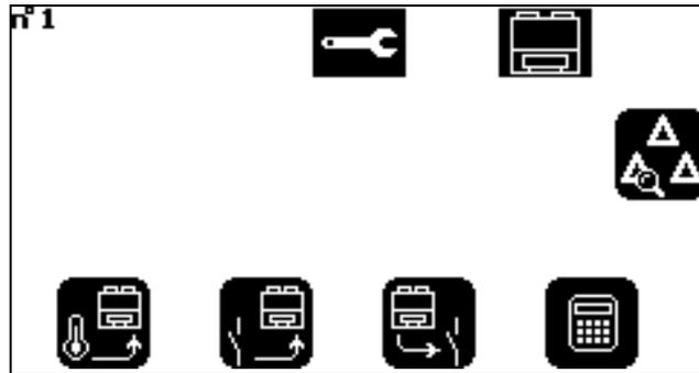
This screen gives access to the values of analogue inputs, logic inputs, TOR outputs, fault counters, and other variables relating to the entire machine (not related to a specific refrigeration circuit). Each variable is identified by its mnemonic.
