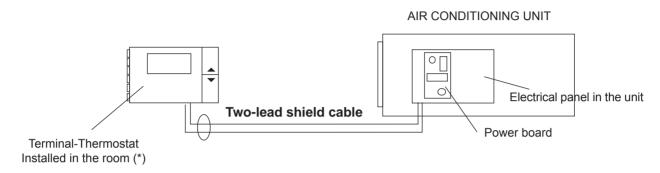
(\*)If a remote sensor is requested as an option, the terminal-thermostat can be installed in a different place from the room to be conditioned
