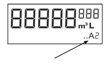
The figure after the "A" indicates how many times the meter has been adjusted or reset. In a completely new meter both of these indicators will be switched off.
