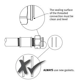
The piping must be parallel and fit the meter.
