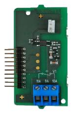
Figure 28. Galvanically separated output module (Y=2).
