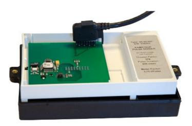
Figure 45. Location of the eight-pole plug in Pulse Divider 66-99-607.
