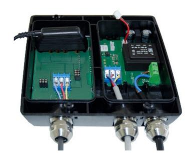
Figure 46. Location of the four-pole plug in Pulse Divider 66-99-907.
