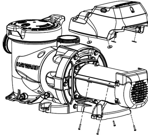
**Note:** Motor leads must be disconnected prior to removing drive, and reconnected when new drive is mounted. Take care to ensure that the motor leads are not pinched between the drive enclosure and the motor during assembly. The drive mounting screws must be tightened to 30 inch-pounds.
