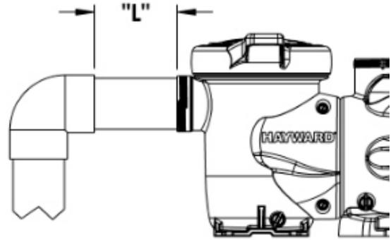
**Note:** It is recommended that a minimum length of straight piping (shown as "L" in above diagram), equivalent to 5 pipe size diameters, be used between the pump suction inlet and any plumbing fittings (elbows, valves, etc.).
