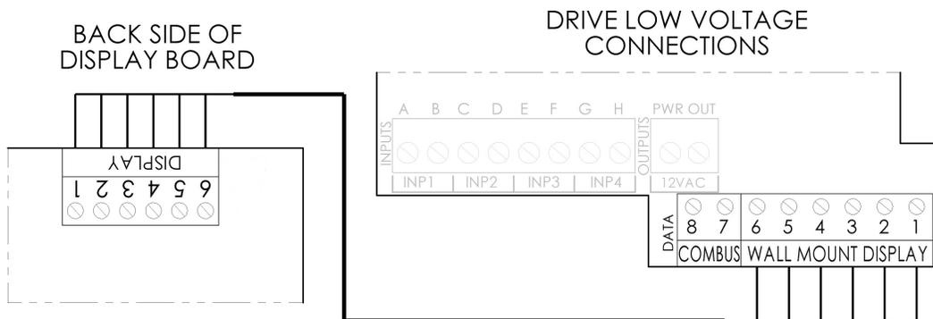
Connection wire must be rated for a minimum of 300V, and may be up to 500 feet in length. Use removable 6-position terminal block connectors for wiring connection to display and motor drive board taking care to note the wire colors and corresponding numbers next to the connectors. Do **not** connect to the upper input terminals shown as light gray above.
