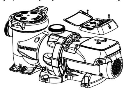
Figure 4.12-1: Removing the Digital Control Interface for Wall Mounting
