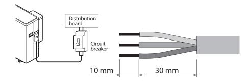
• Use a circuit breaker with a 3 mm clearance of air gap between the contacts.
