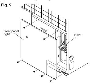
(3) Open the piping and connection cord knockout holes of the desired direction with nippers, etc. After opening a hole in the center of bush, pierce with connection cord. (Rear, Right and Left wiring)
