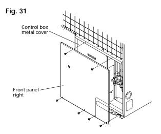
(2) Remove control box metal cover and connect the power supply cord and the outdoor unit connection cord wire at the indoor unit.
