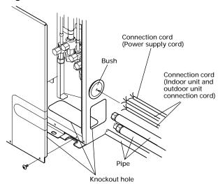
(4) Connect the piping and connection cord from the mounting holes.
