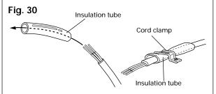
Use VW-1, 0.5 to 1.0 mm thick, PVC tube as the insulation tube.
