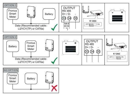
\*) The R 120 Ohm terminating resistor is supplied with the Fronius Smart Meter
