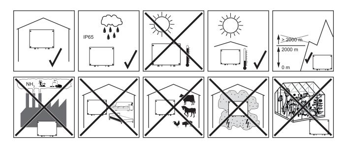
Possible assembly positions when using outdoors:
