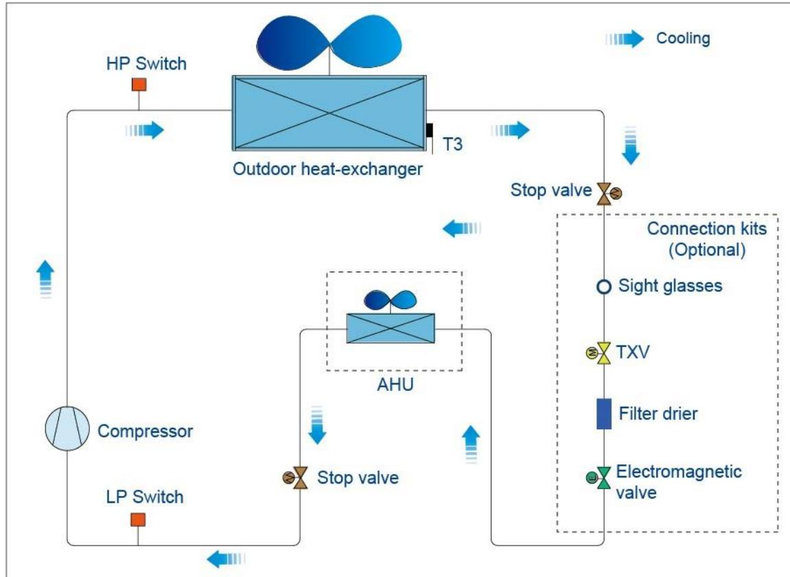
SCCU36C1BR, SCCU48C1BR, SCCU60C1BR, SCCU75C1BR, SCCU96C1BR, SCCU120C1BR, SCCU150C1BR
