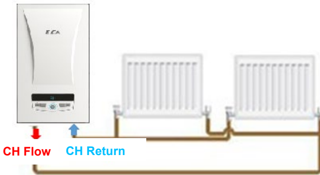
Figure 8. CH Device Installation Scheme
