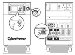
Step 1: Turn off the POWER SW, Output Selector and the BATTERY SW.
