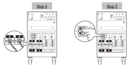
5. Connect the batteries to the BATTERY INPUT. (Step4)
