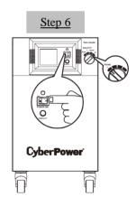
11. When the external battery needs to be maintained or replaced, remember to turn the machine off. Once off, remove the AC power source and switch off the BATTERY SW. before maintenance or replacing the batteries. When the work is complete, please start from Step 1 to re-install the machine.
