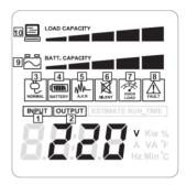
3. NORMAL MODE Icon: This icon will illuminate when the EPS is working under normal conditions.
