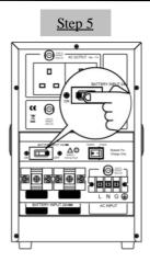
5. Connect the batteries to the BATTERY INPUT. (Step4)
