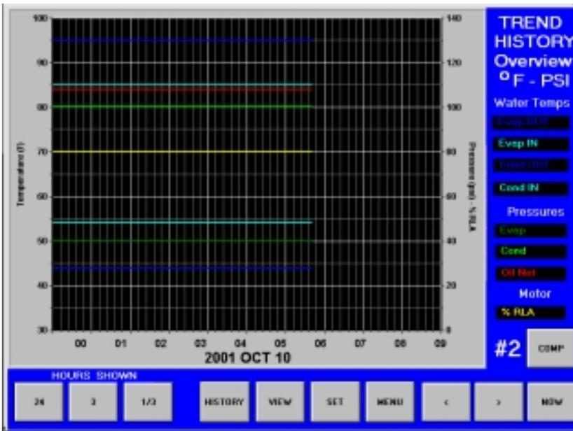
Ever wonder how your chiller performed last week? Were you holding chilled water temperature? What kind of cooling load did the chiller have? The McQuay MicroTech II can reach back in the past, thanks to its huge memory, and plot water temperatures, refrigerant pressures, and motor load. These values can also be downloaded through a convenient floppy drive, located right in the Interface Panel, and pasted into a spreadsheet for further evaluation.
