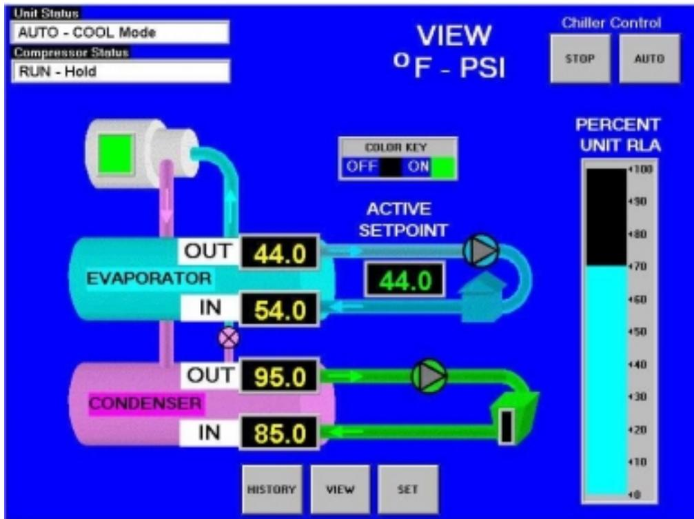
The Home Screen shown above is usually used as the primary viewing screen. It gives real time data on unit status, water temperatures, chilled water set point and motor amp draw. In other words it very clearly answers the vital question-is the chiller operating properly?
