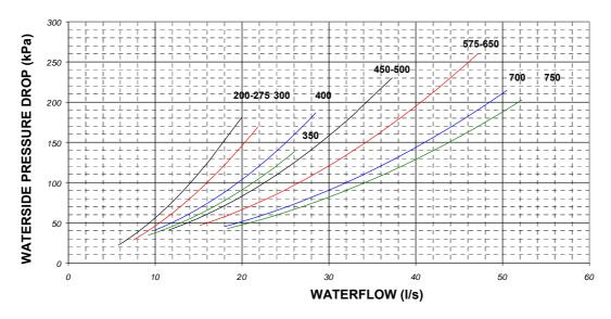
**WATERSIDE PRESSURE DROPS** (20% Ethylene Glycol Concentration)
