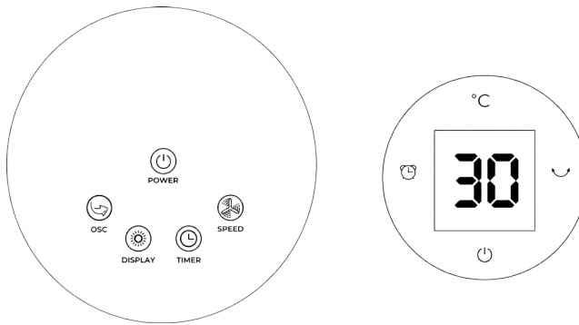
Control panel and display
