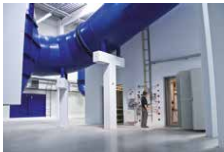
Installation type A according to ISO 5801
