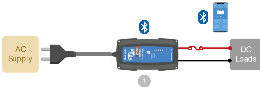
Battery charger used as a power supply.
