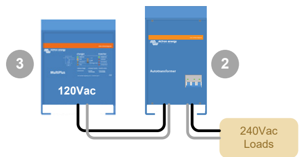
Autotransformer stepping up a single phase 120Vac supply into a single phase 240Vac supply
