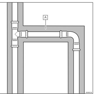
Chased pipes must not be in direct contact with the plaster, but wrapped in a pad of elastic material, such as glass wool or plasticfoam (A). Thus fitted, soundproofing requirements can also be satisfied, but always refer to local guidelines and regulations.
