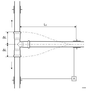
The diagram for Z-compensators also applies here.
