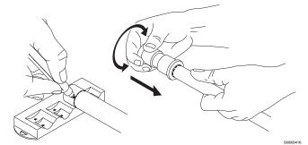
2. Press the fitting onto the pipe with the appropriate tool and visually check the result.
