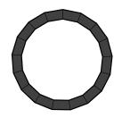
If the fitting is not pressed, the particular profile of the o-ring identifies the irregular condition, both during the seal test and visually/audibly, through leaking of water or air. This characteristic is commonly known as "unpress - untight". After the fitting has been pressed, the o-ring easily closes all the flows, ensuring the hermetic seal as with the traditional type.
