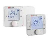
Used together with c.pCO mini programmable controllers. The terminal is equipped with a built-in temperature gauge. Concealed and wall-mounted versions are available. The terminal requires a power supply for operation.
