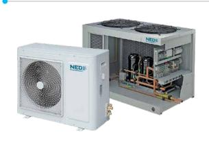
Condensing units are designed for the preparation of refrigerant transferred to the heat exchanger of the inner unit or to the section of direct evaporation in the air conditioning system. Non-reversing singe-circuit (NSK and ND-SPL) and twin-circuit compressor-condensing (NSK) with axial fans and rotary/scroll compressors in 27 standard sizes with a capacity from 2 to 255 kW. Outdoor design of the units. Used refrigerant: R410A.
