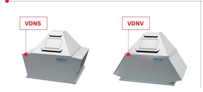
Roof fans with air exhaust to the sides/ up are designed to move smoke-air mixtures with a temperature of 400°C or 600°C for 120 minutes in case of fire.
