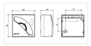
Electrical contact capacity = 16(2,5) A / 250 Vac Regulation range = 5°÷30°C Differential = 1K Insulation class = II Protection rating = IP20 Max. tolerance temperature = 50°C Connection = 2 wires Output = changeover switches Operating mode: On/Off or Summer/Winter System: heating/air conditioning Certifications: CE, ENEC03, EAC
