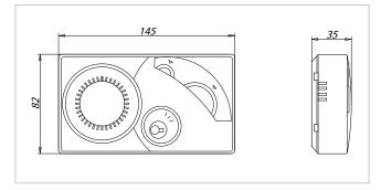
Electrical contact capacity = 5(1) A / 250 VacTemperature range =  $10^{\circ} \div 30^{\circ}\text{C}$ Differential = 0.5 K Insulation class = II Protection rating = IP20 Max. room temperature =  $50^{\circ}\text{C}$ Power supply = 2 x 1.5V-LR6 AA batteries Operating mode: Manual / Automatic Heating system Form of control: TPI (optional) Certifications = CE, ENEC03
