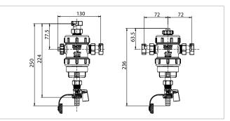
Max pressure = 3 bar Max. temperature = 0 ÷ 90°C Compatible fluids = Water and non-aggressive fluids Connections: G3/4" ISO228/1 female swivel captive nut hose fitting Ø15 mm Certifications = CE
