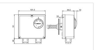
Electrical contact capacity = 10 (2,5) A / 250 Vac Adjustable temperature FAN = 0°/60°C Internal adjustable temperature LIM = 30°/120°CProtection rating = IP40 Max. head temperature = 80°CMax. bulb temperature = 150°CCertifications = CE, ENEC03, EAC
