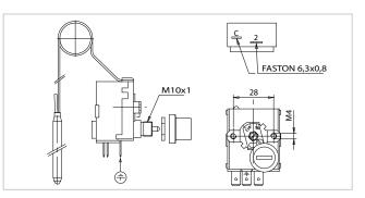
Switches = interrupted due to temperature increase Max. head temperature =  $85^{\circ}$ C Copper bulb =  $125^{\circ}$ C Copper bulb = Ø 6,5 x 95 mm Min. capillary curvature radius = 5 mm Certifications = CE, ENECO3, EAC, UL, CSA
