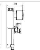
WATERLINK WTL6 is a hydraulic separation module between two heat generators powered by different energy sources. The most typical appliance is that between a thermo-fireplace (or a thermo-heater) and a gas boiler. When handling heat produced by the biomass source, the module disables the traditional boiler and activates the 3-way valve to send hot water to the domestic heating system. Otherwise the 3-way valve is not enabled, allowing the gas boiler to meet the required heating needs.
