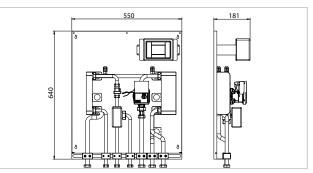
Supply voltage = 230 V / 50 HzMax. absorbed power = 100 WWater temperature probe = NTC 1% Operating water temperature =  $0/95^{\circ}\text{C}$ Max. water probe temperature =  $150^{\circ}\text{C}$ Working room temperature =  $0/60^{\circ}\text{C}$ Storage temperature =  $0/60^{\circ}\text{C}$ Max. heating fluid pressure = 3 bar Max. fluid pressure ACS = 6 bar Protection rating = IPX4D Certifications = CE
