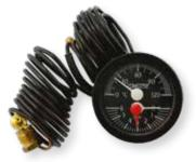
Range of liquid expansion thermomanometers and connection for manometer. Particularly suitable for appliance on boilers, fireplaces, heaters and home appliances. Available in a round version with different measuring ranges and colours (customisable typeface and dials). Working range =  $0/120^{\circ}$ C - 0/6 bar Casing = plastic Max. body temperature =  $70^{\circ}$ C Certifications = CE, EAC
