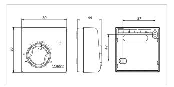
Electrical contact capacity = 16(2,5) A / 250 Vac Regulation range = 5°÷30°C Differential = 1K Insulation class = II Protection rating = IP20 Max. tolerance temperature = 50°C Connection = 2 wires Output = changeover switches Operating mode: On/Off or Summer/Winter System: heating/air conditioning Certifications: CE, ENEC03, EAC
