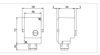
Temperature limiter pre-regulation =  $60^{\circ}$ C Regulation range =  $40^{\circ}$ ÷70°C Tolerance = 0-10K Manual reset Reset temperature =  $-25K \pm 8K$  range Max. head temperature =  $55^{\circ}$ C Electrical contact capacity = C-1: 0,5 A / 250 Vac C-2: 10(2,5) A / 250 Vac Protection rating = IP40 Certifications = CE, ENEC03, EAC
