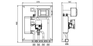
Supply voltage = 230 V / 50 Hz Max. absorbed power = 100 W Water temperature probe = NTC 1 % Operating water temperature = 0/95°C Max. water probe temperature = 150°C Working room temperature = 0/60°C Storage temperature = 0/60°C Max. fluid pressure = 3 bar Protection rating = IPX4D Certifications = CE
