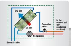
If continuous unit operation is required for protection against faults, the **TREF Dual Cooling** range is also available in a dual circuit design - allowing for server room refrigeration even in the event of either circuit failure.
