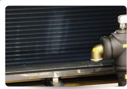
All models in the **TREF Dual Cooling** range feature standard heat exchange coils with hydrophilic coating. This special coating - together with an adequate adjustment of air through-flow speeds - helps condensate collection during the dehumidification process, avoiding dripping on the inside and outside of the unit.
