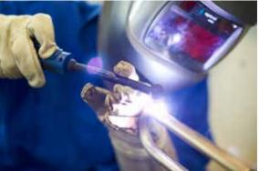
Modern technology also in detail: Orbital welding enables consistently high levels of seam quality for our products.
