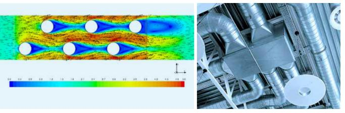
By means of thermodynamic simulations, the CABERO engineers determine the ideal flow speed to prevent flow separation drops and escaping moisture.
