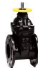
Series 15/78 Flanged gate valve with ISO top flange Short DIN F4 DN50-400 PN10/16 Ductile iron With external PUR coating
