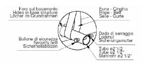
Use ropes or belts long enough to extend beyond the height of the unit and place spacer bars and boards on the top of the unit to avoid damaging the sides and top of the unit itself. The rectangular holes are provided for the attachment of vibration damping supports (optional).
