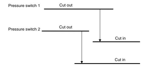
...where <u>pressure switch 1</u> is set at the "PS" (maximum admissible pressure) of the system, while <u>pressure switch 2</u> will have the setting =  $PS \times 0.9$  in accordance with the reference technical standard.
