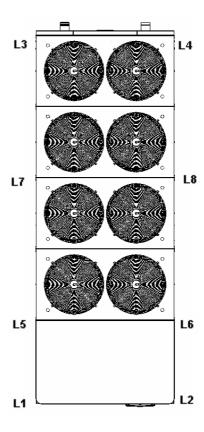
This drawing illustrates the points of the machine for which the **weights for the basic chiller and heat pump models** have been calculated. The values are shown in the following tables.
